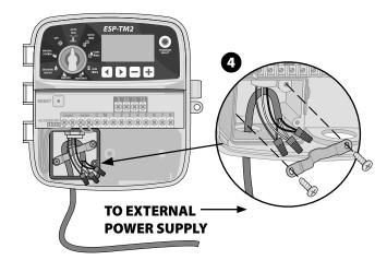
Power Wiring Connections (120VAC)
