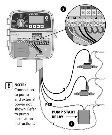
NOTE: The ESP-TM2 controller DOES NOT provide I power for a pump. The relay must be wired according to manufacturer instructions.
