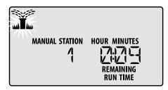
• To cancel manual watering, turn the dial to **OFF** for three seconds until the screen shows OFF.
